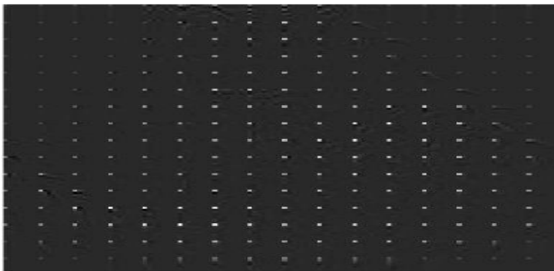
Figure 5: Two dimensional DCT coefficients of given image
